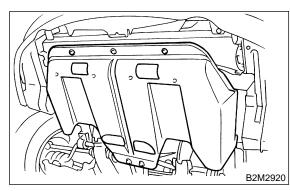
3) Remove drain cock to drain engine coolant into container.
