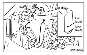
Attach radiator cap and reservoir tank cap properly.
