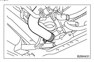
5) Remove thermostat cover and gasket, and pull out the thermostat.
