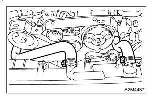
11) Remove radiator sub fan motor assembly.
