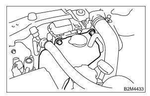
10) Disconnect radiator inlet hoses from radiator.
