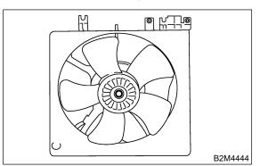
3) Remove screws which install fan motor onto shroud.
