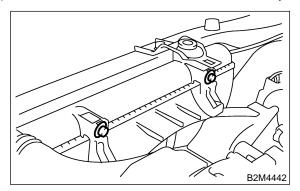
12) Remove radiator main fan motor assembly.
