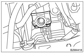
3) Install EGR pipe to EGR valve and cylinder head.
