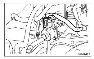
2) Install EGR valve to intake manifold.
