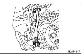
5) Remove EGR valve from intake manifold.
