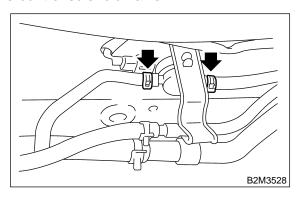
6) Remove pressure control solenoid valve from bracket.
