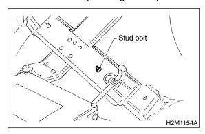
9) Use engine grounding terminal or engine proper as the grounding point to the body when measuring voltage and resistance in the engine compartment.
