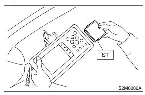
4) Connect test mode connector at the lower portion of instrument panel (on the driver's side), to the side of the center console box.
