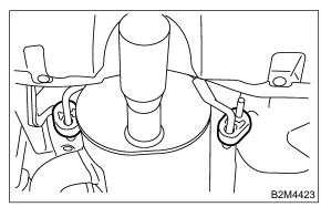
3) Remove front rubber cushion, and detach muffler assembly.
