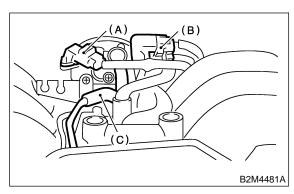
7) Disconnect throttle position sensor connector.
