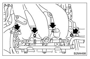
28) Remove intake manifold.
