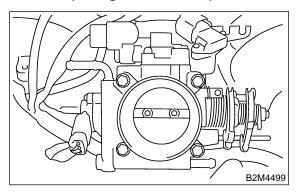
17) Connect connectors to throttle position sensor.
