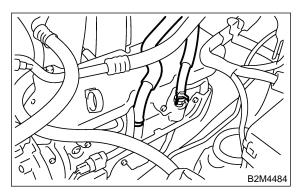
14) Disconnect engine coolant hose from throttle body.
