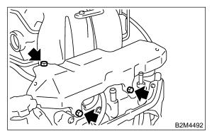
9) Install ground cable to fuel pipe protector LH.
