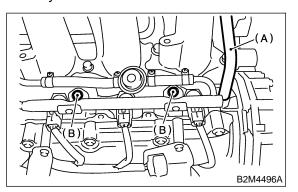
27) Remove bolts which holds intake manifold onto cylinder heads.
