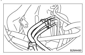
12) Connect engine ground terminal to intake manifold.
