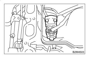
9) Install purge control solenoid valve.
