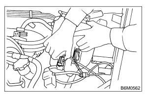
21) Install washer tank on body.
