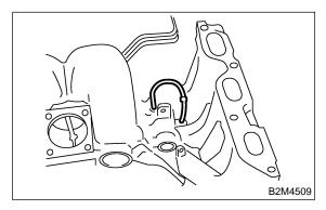
2) Install fuel pipe and injector pipe assembly.
