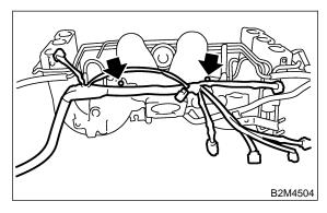
13) Remove PCV pipe from intake manifold.
