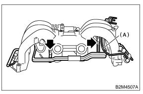
4) Install air assist and purge pipe assembly.
