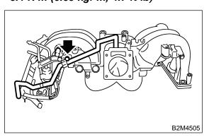
6) Install engine harness assembly to intake manifold.
