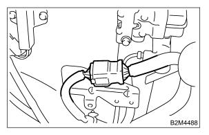
18) Disconnect engine ground terminal from intake manifold.
