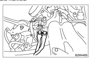
19) Disconnect fuel hoses from fuel pipes.
