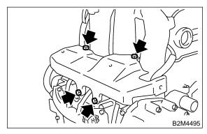
5) Install ground cable to fuel pipe protector RH.
