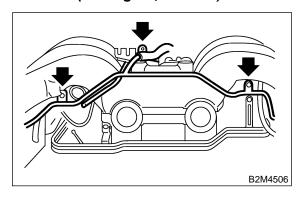
5) Install PCV pipe to intake manifold.
