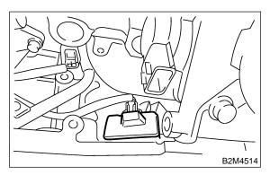
5) Remove bolt which install crankshaft position sensor to cylinder block.
