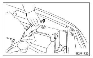
Remove air intake chamber. <Ref. to IN(H6)-6, REMOVAL, Air Intake Chamber.>
