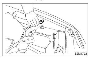
2) Disconnect connector from intake manifold pressure sensor.
