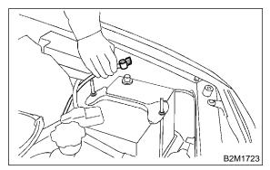
2) Disconnect connector from rear oxygen sensor.
