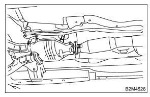
3) Connect connector to rear oxygen sensor.
