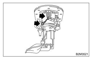
3) Pushing the pawls with a screwdriver, remove fuel meter unit by pulling it downwards.
