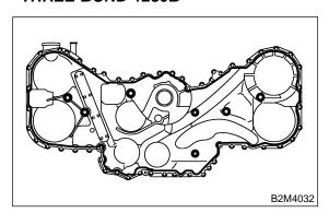
3) Install front chain cover. Temporarily tighten the bolts.
