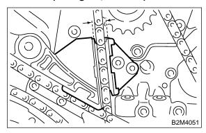
(8) After checking the matching marks on each sprocket and corresponding timing chain are aligned, pull stopper pin out of chain tensioner.
