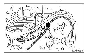
Remove chain guide. (Left-hand between cams)
