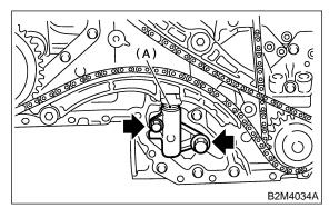
4) Remove chain guide. (Right-hand between cams)
