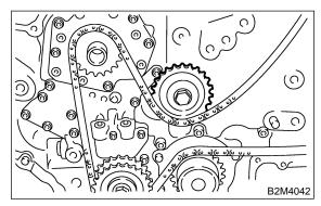
(4) Install chain guide. (Left-hand between cams)
