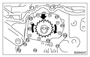
5) Install the idler sprocket. (Lower)
