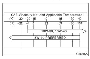
The proper viscosity helps vehicle get good cold and hot starting by reducing viscous friction and thus increasing cranking speed.
