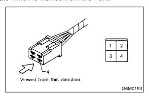
• The number of poles or pins, presence of a lock, and pin number of each terminal are indicated in the sketch of each connector. In the sketch, the highest pole number refers to the number of poles which the connector has. For example, the sketch of the connector shown in figure indicates the connector has 9 poles.
