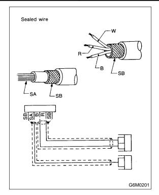
• The wire color code, which consists of two letters (or three letters including Br or Lg), indicates the standard color (base color of the wire covering) by its first letter and the stripe marking by its second letter.
