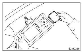
(2) Connect Subaru Select Monitor to data link connector.
