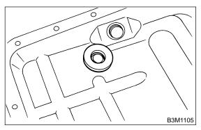
5) Apply proper amount of liquid gasket to the entire oil pan mating surface. **Fluid packing:**
