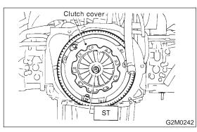
3) Remove clutch cover and clutch disc. <Ref. to CL-7 REMOVAL, Clutch Disc and Cover.>
