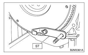
2) Tighten the flywheel attaching bolts to the specified torque.
