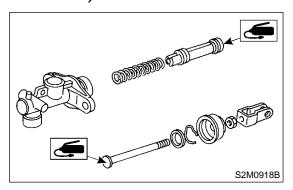
2) To assemble the master cylinder reverse the sequence of disassembly procedure.
