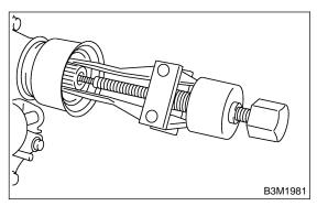
7) Using ST, install the oil seal. ST 498057300 INSTALLER
