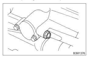
3) Install the manual transmission assembly to vehicle. <Ref. to MT-30 INSTALLATION, Manual Transmission Assembly.>
