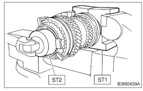
3) Remove 5th-Rev sleeve and hub assembly, baulk ring, 5th drive gear and needle bearing (32  $\times$  36  $\times$  25.7).
