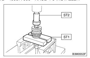
6) Using ST1 and ST2, install the 5th gear thrust washer and 5th needle bearing race onto the rear section of transmission main shaft.
