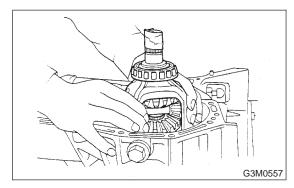
2) Install main shaft assembly. <Ref. to MT-54 INSTALLATION, Main Shaft Assembly.>
