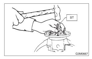
4) Pull out pinion shaft, and remove differential bevel pinion and gear and washer.
