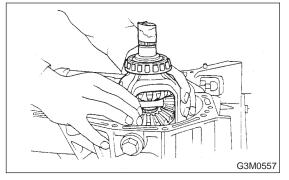
7) Remove differential side retainers using ST. ST 499787000 WRENCH ASSY
