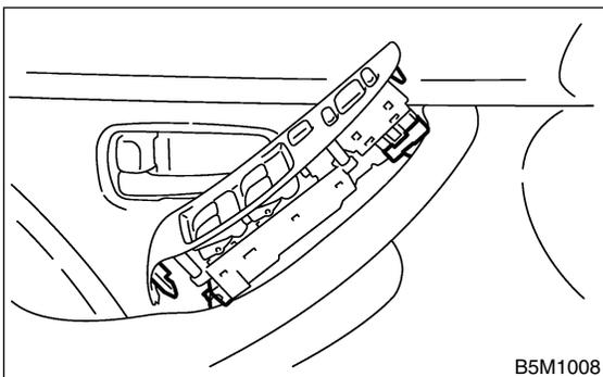
4) Remove three screws and clips.
