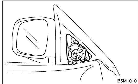
6) Remove seven clips of trim panel using clip remover to remove trim panel.
