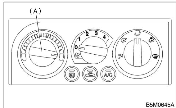
11) Set temperature control switch (A) to "FULL HOT" and then disconnect temperature control cable from bottom of heater unit. (Manual A/C equipped model)
