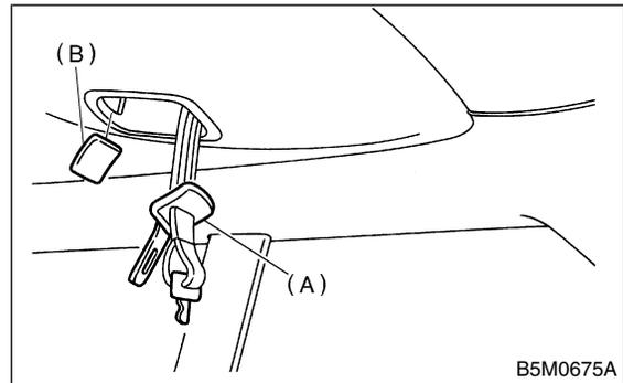
13) Remove clips and then remove roof trim.
