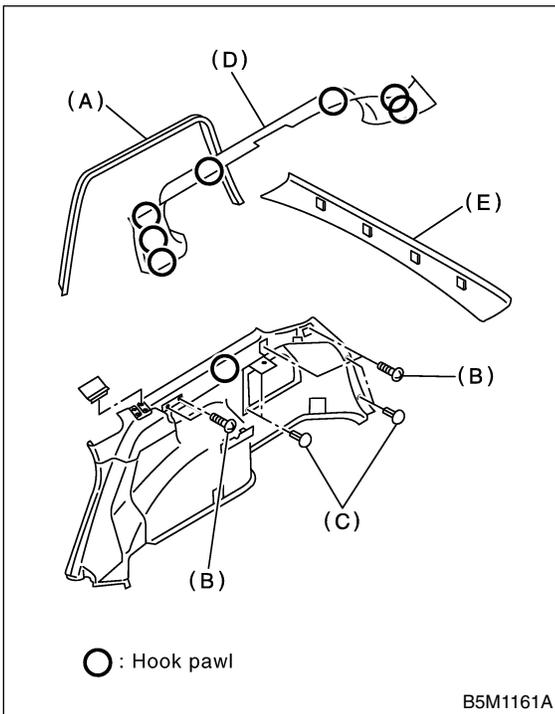
12) Remove cover (B) while detaching snap lock carefully. Put the rear center seat belt tongue (A) out to the other side of the trim through the hole.
