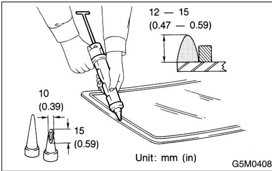
12) Apply adhesive to glass end surface as shown.
