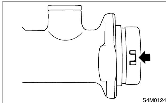
4) Using pliers, install C-ring in its groove. (With VDC)
