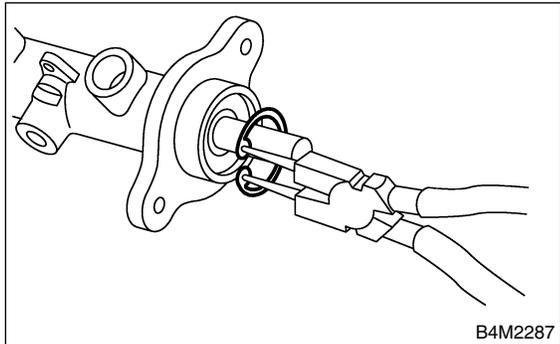
5) Extract primary piston assembly and secondary piston assembly.
