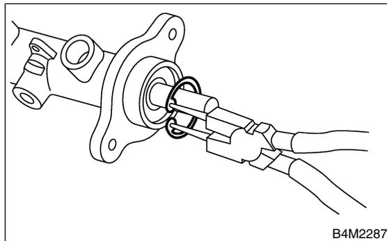
5) Install seal to reservoir tank.
