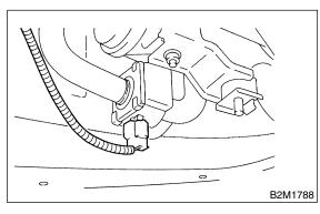
6) Remove nut which installs drain filter and drain valve brackets on body, and remove them as a unit.
