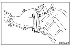
2) Install front and center exhaust pipes. <Ref. to EX-6, INSTALLATION, Front Exhaust Pipe.>
