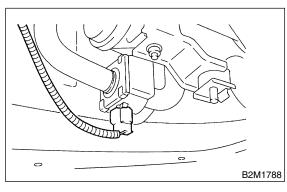
6) Remove bolt which installs air filter and drain valve brackets on body.
