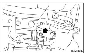
7) Disconnect evaporation hose and remove drain valve.
