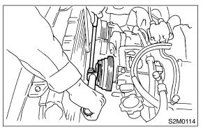
10) Remove water pump. <Ref. to CO-14 REMOVAL, Water Pump.>
