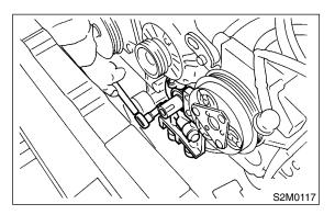
13) Remove oil pump by using flat bladed screw-driver.
