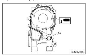
3) Apply a coat of engine oil to the inside of the oil seal.
