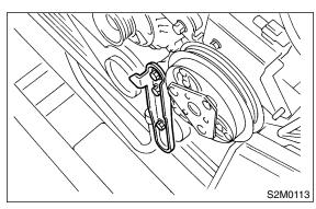
9) Remove crankshaft pulley by using ST. ST 499977100 CRANKSHAFT PULLEY WRENCH
