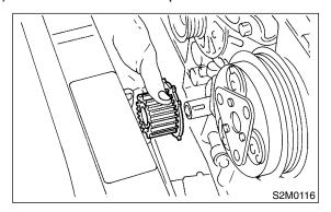
12) Remove bolts which install oil pump onto cylinder block.
