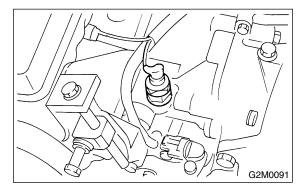
4) Install generator on bracket. <Ref. to SC-15, INSTALLATION, Generator.>
