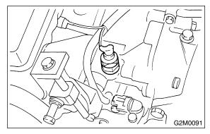
3) Remove oil pressure switch.
