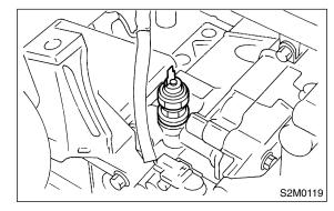
3) Connect terminal of oil pressure switch.
