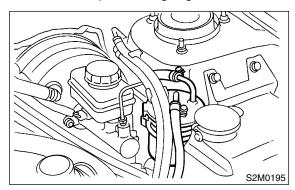
4) Connect connector of fuel pump relay.
