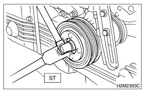
3) Remove crankshaft pulley.
