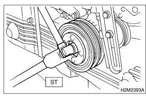
3) Confirm that the tightening angle of the crankshaft pulley bolt is 65 degrees or more. If not, conduct the following procedures (1) through (4).
