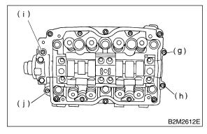
(3) Install valve rocker assembly.
