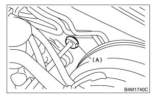
11) Pull out the cable from the toe board hole.12) Disconnect accelerator cable bushing from accelerator pedal lever.
