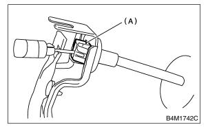
14) Separate accelerator cable and bracket.
