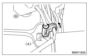
2) Disconnect the positive (+) cable after disconnecting the negative (-) cable of battery.
