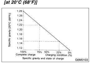
2) Measuring the specific gravity of the electrolyte in the battery will disclose the state of charge of the battery. The relation between the specific gravity and the state of charge is as shown in figure.
