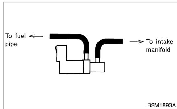
4) Remove bolt which installs purge control solenoid valve onto intake manifold.
