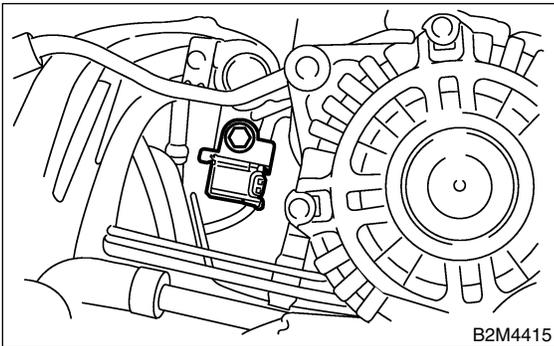
5) Take out purge control solenoid valve through the bottom of the intake manifold.
