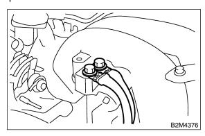
10) Use TCM mounting stud bolts at the body head grounding point when measuring voltage and resistance inside the passenger compartment.
