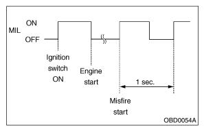
4) When ignition switch is turned to ON (engine off) or to "START" with the test mode connector connected, the MIL blinks at a cycle of 3 Hz.
