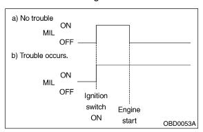
3) If the diagnosis system senses a misfire which could damage the catalyzer, the MIL will blink at a cycle of 1 Hz.
