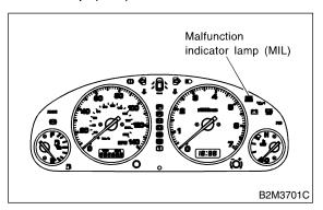
2) After starting the engine, the MIL goes out. If it does not, either the engine or the emission control system is malfunctioning.
