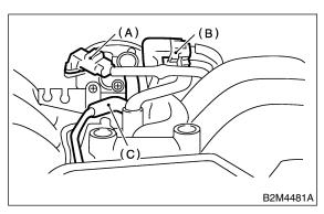
7) Disconnect throttle position sensor connector.
