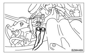
13) Connect engine harness connectors to bulk-head connectors.
