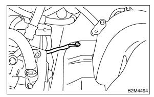
6) Install the bolt (B) which holds fuel injector pipe RH onto cylinder head.
