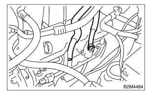
14) Disconnect engine coolant hose from throttle body.
