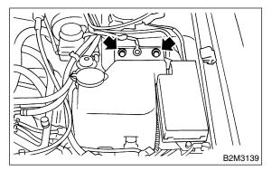
9) Disconnect connector from front window washer motor.
