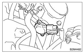
18) Connect connectors to intake manifold pressure sensor (A) and idle air control solenoid valve (B).
