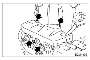
26) Disconnect air assist hose (A). Remove the bolt (B), which holds fuel injector pipe RH onto cylinder head.
