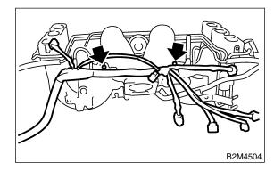
13) Remove PCV pipe from intake manifold.
