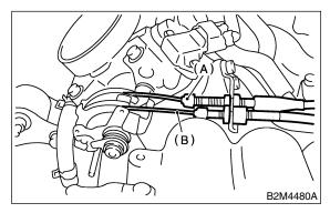
7) Remove power steering pump and tank from brackets.
