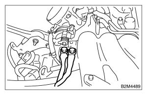
19) Disconnect fuel hoses from fuel pipes.
