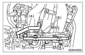
24) Remove ground cable from fuel pipe protector RH.
