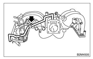
6) Install engine harness assembly to intake manifold.
