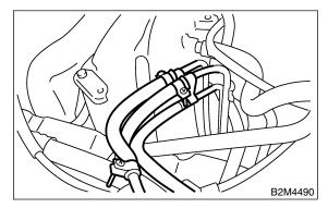
20) Remove ground cable from fuel pipe protector LH.
