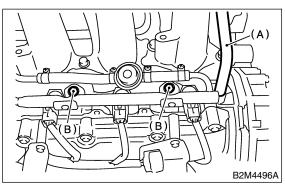
27) Remove bolts which holds intake manifold onto cylinder heads.
