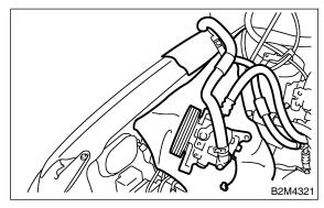
8) Remove two bolts which install washer tank on body.
