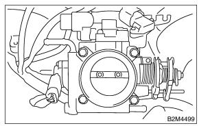
17) Connect connectors to throttle position sensor.
