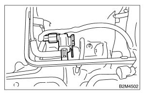
11) Connect hoses to purge control solenoid valve.
