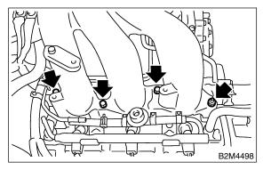
2) Install the bolt (B), which holds fuel injector pipe RH onto cylinder head.
