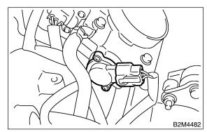
2) Disconnect connectors from intake manifold pressure sensor (B) and idle air control solenoid valve (A).
