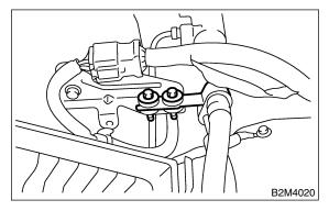
(3) Remove bolts which install power steering pump bracket.
