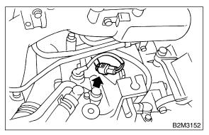
(5) Remove power steering tank from the bracket by pulling it upward.
