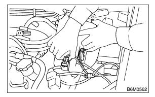
21) Install washer tank on body.
