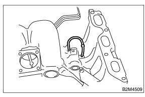
2) Install fuel pipe and injector pipe assembly.
