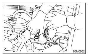
11) Disconnect rear window glass washer hose from washer motor, then plug connection with a suitable cap.
