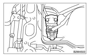
9) Install purge control solenoid valve.
