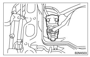
12) Remove engine harness assembly from intake manifold.
