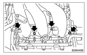
28) Remove intake manifold.
