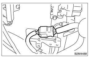
18) Disconnect engine ground cable from intake manifold.
