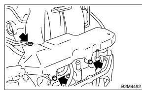
9) Install ground cable to fuel pipe protector LH.
