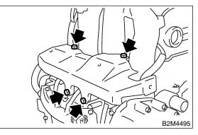
5) Install ground cable to fuel pipe protector RH.
