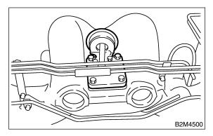
15) Connect hoses to induction valve control solenoid.
