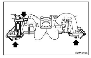
17) Remove induction valve vacuum hose from intake manifold.
