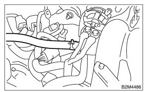
15) Connect engine coolant hose to throttle body.
