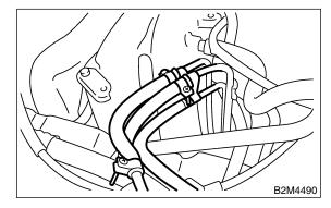
12) Connect engine ground cable to intake manifold.
