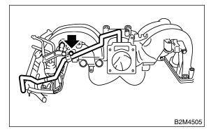
14) Remove air assist and purge pipe assembly.
