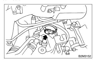
(5) Remove power steering tank from the bracket by pulling it upward.
