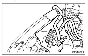
6) Remove ground cable from fuel pipe protector RH.
