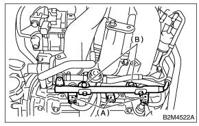
13) Remove fuel injector while lifting up fuel injector pipe.
