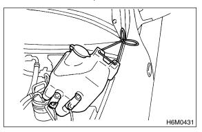
9) Remove ground cable from fuel pipe protector LH.
