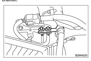
(3) Remove bolts which install power steering pump bracket.
