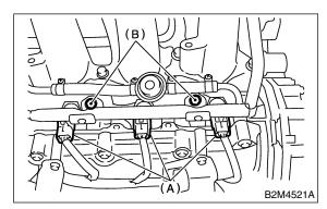
10) Remove fuel injector while lifting up fuel injector pipe.
