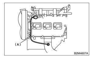
6) Apply SUBARU CRC or its equivalent to threaded portion of front oxygen (A/F) sensor, and leave it for one minute or more.
