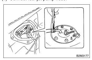
(2) Connect connector from fuel sub level sensor.
