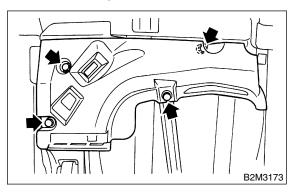
5) Drain fuel from fuel tank. Set a container under the vehicle and remove drain plug from fuel tank.
